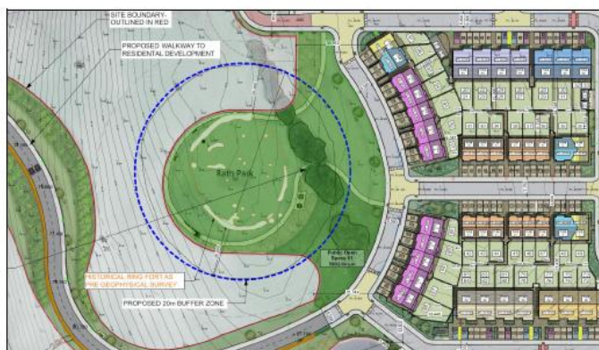
FIGURE 2: Proposed development plan overlaid with geophysical survey results for CV020-057 which informed the proposed 20m construction exclusion zone (blue)
