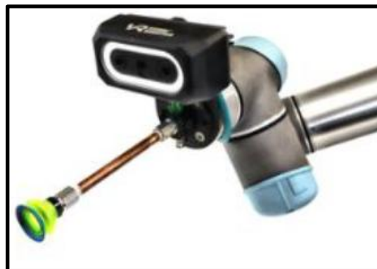
VIM-303 Camera and Suction Gripper mounted on Universal Robots arm
