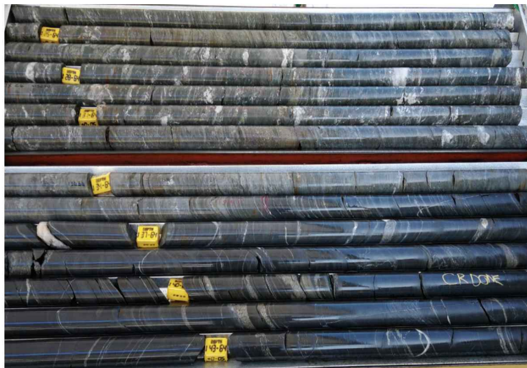
Figure 4. Drill core showing lithological units of the SF3 ore body
