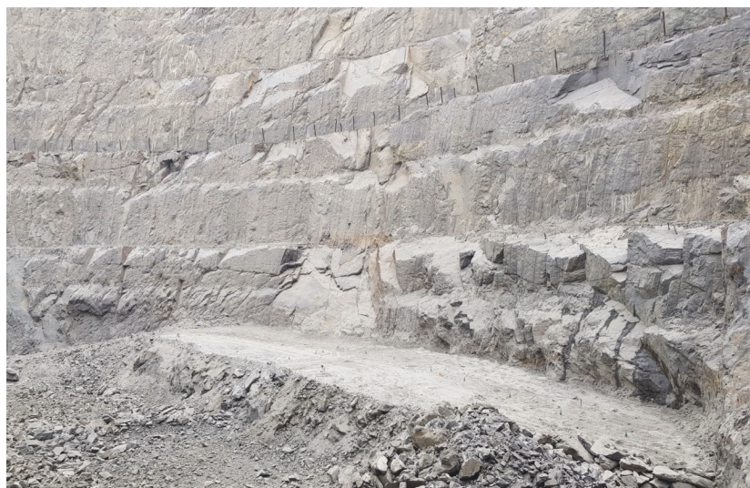
Figure 4 Example of west wall, mined to RL 908, batters undercut by J1 joints, with rockfalls and batter failure, and supported by shear pins (right of photograph)
