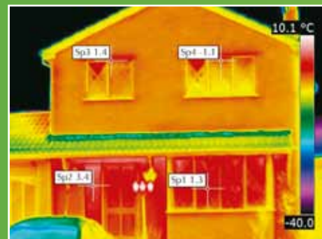
The warmest areas seen here in red show where heat is being lost from the building.
