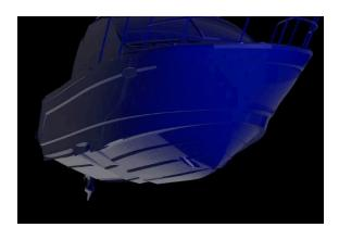
Our outboard engine boats incorporate an advanced hull design to optimize efficiency, performance, and maneuverability. These features include an innovative combination of a steep deep-V hull for a smooth ride, a keel pad for planing stability, and reversed chines for quick planing and reduced cornering roll. The double-stepped hull increases efficiency and performance and reduces fuel consumption.
