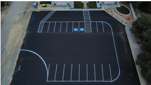
Multi-tenant retail lot. Custom layout with curved striping, two ADA bays, and a bus lane.
