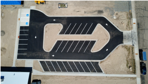
New-build retail lot. Custom layout from scratch — striping, arrows, and two van-accessible ADA bays.
