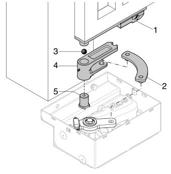
**06.** Place the gate leaf on the release lever and secure it with bolts (a) or a strong weld (b)
