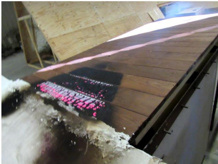
The test burner flame was cut-off at 10 minutes. The flames on the sample self-extinguished at 10 seconds after the test burner flame was cut-off.
