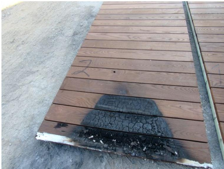
Post test photo of test #2. Deck removed from the test frame.
