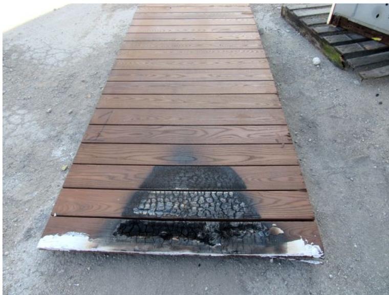
Post photo of test #1. Deck removed from the test frame.
