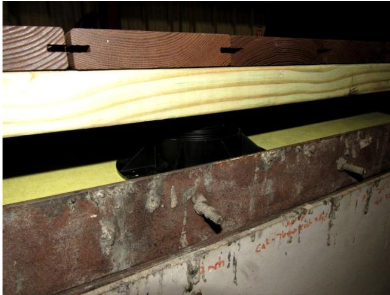
Side view: ASTM E 108 steel test frame, DensGlass® Sheathing, Plastic leveling pedestals, 2 x 4 board runners and the Thermally Modified Ash Decking Panels
