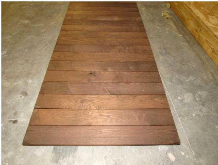
Finished Surface of Thermally Modified Ash Decking Panel
