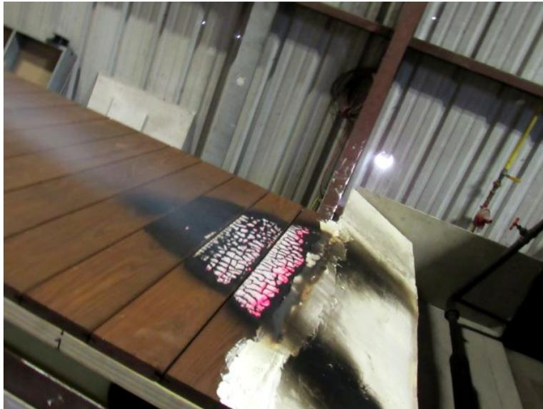
**The test burner flame was cut-off at 10 minutes. The flames on the sample self-extinguished at 7 seconds after the test burner flame was cut-off.**
