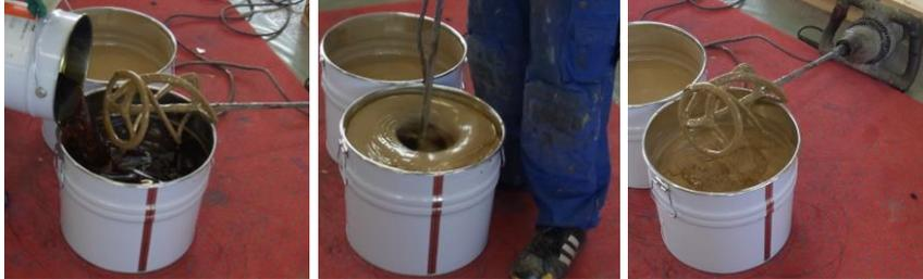
Mixing of the 2-component PU adhesive
