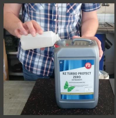
Open both components and pour component B (hardener) completly into the canister.
