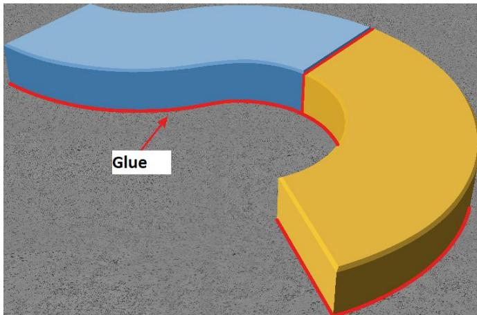
2. The EUROFLEX® C & S Blocks may be used without adhesion to the substructure and can be installed directly in a fresh concrete bed (dimensionally stable at B15). For this purpose, several galvanized hex lag screws (10 × 200 mm, minimum embedment 70 mm) are driven into the rubber and the screw heads are embedded in the fresh concrete. Glue or join the joints between the block steps.
