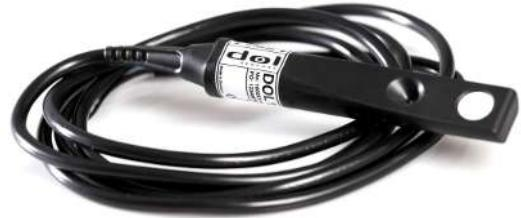
DOL 114 is a high-precision humidity sensor for measuring relative humidity and temperature. It is intended for application in livestock houses but is also well suited for a number of industrial applications.
