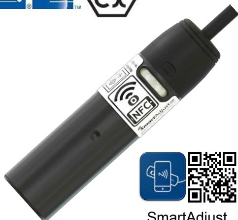
iDOL 46R capacitive relay sensor series is designed for general detection of feed, grain and solids. Certified according to ATEX directive 2014/34/EU, IECEx for operation in hazardous, potentially explosive dust atmospheres. Classified as equipment for use in atmospheres with continuous presence of explosive dust with an ignition temperature above 85 °C.
