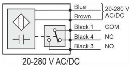
Supply voltage is connected to the blue and brown wire.
