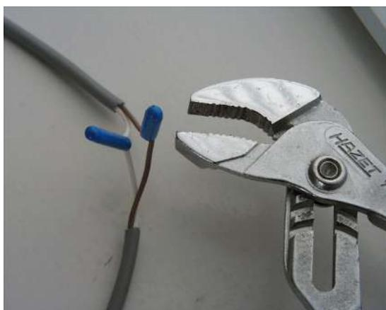
Splices must be done very carefully by means of the enclosed blue silicone sleeves. Tracking current between conductors will result in indication error. Connection terminals will create problems in the course of time and should therefore not be used.
