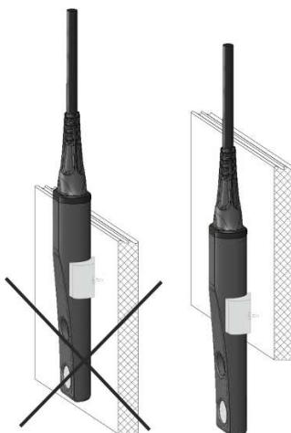
For optimum mounting of the sensor, use mounting clip or mount it free-hanging in the cable.
