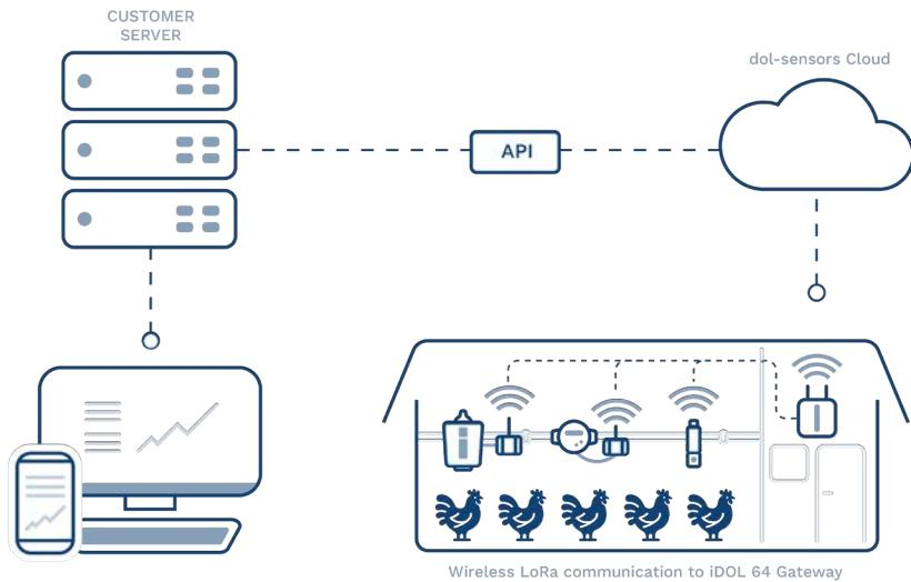
Data is sent wirelessly from the sensors or via a LoRa converter to the iDOL 64 Gateway. The gateway sends the data to the dol-sensors Cloud and through the API directly to your server every hour around the clock. Save the data on your server to keep it as the data is deleted from the dol-sensors Cloud.
