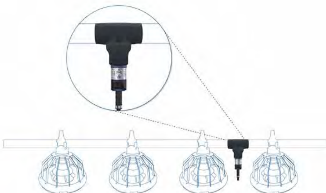
Example of DOL 45 mounted with the T-piece on a 40-60mm tube with conveying system
