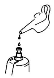
Lubricate regularly (apply a generous amount of oil in the air supply hose 2 to 3 m upstream of the tool). Use only quality air tool oil. If a continuous lubrication unit is used, it should be positioned 3 to 5 m upstream of the tool, or it will not be effective. The oil flow should be set to provide one drop of oil for every 150 liters of free air. If you tend to push the machine hard downwards during work, apply a couple of drops directly into the front part of the tool.
