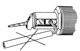
Use the Allen Key to loosen the Blade Lock Screw (4). Insert the blade until you can feel it at the bottom of the mounting slot. Tighten firmly by hand and ensure that the blade is properly clamped. **Use your fingers only.** Overtorquing will break the screw (M7 special)! Mount the blades shown in the figure. It will not work well if mounted upside down, even if you turn the saw around.
