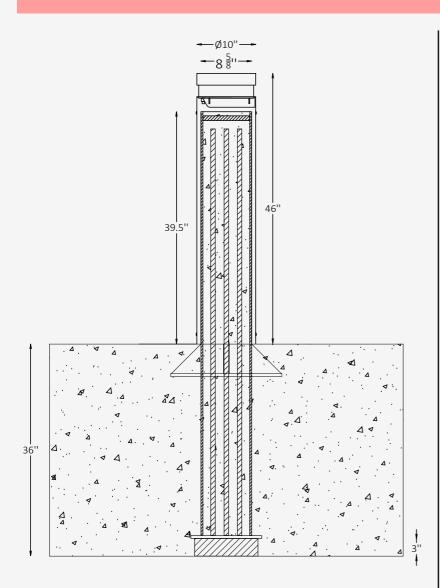
Crash Rating ASTM F2656-07 - M30/P1 Crash Rated Rating Details Certified to meet F2656-07 standards.
