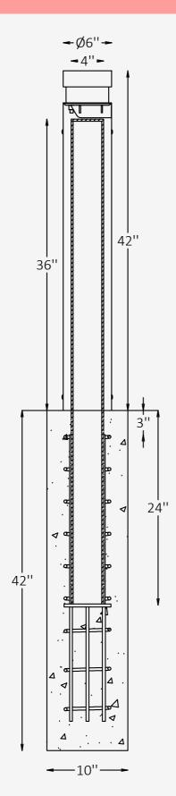
**Crash Rating** ASTM F3016 S10 Crash Rated Certified to meet ASTM F3016. **Rating Details** Tested and proven to stop a 5,000
