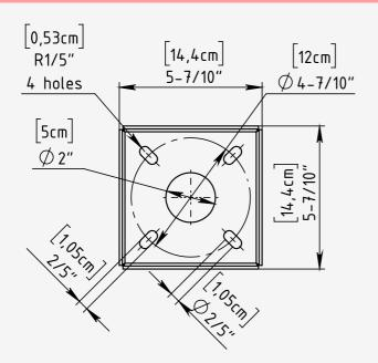
Mounting TypeSurface-mountedBase Plate MaterialStainless SteelBolt Mounting CircleØ: 4-7/10"
