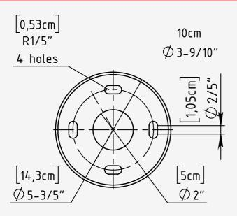
Mounting TypeSurface-mountedBase Plate MaterialStainless SteelBolt Mounting CircleØ: 4-7/10"
