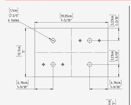
Mounting TypeSurface-mountedBase Plate MaterialStainless SteelBolt Mounting CircleØ: 4-7/10"
