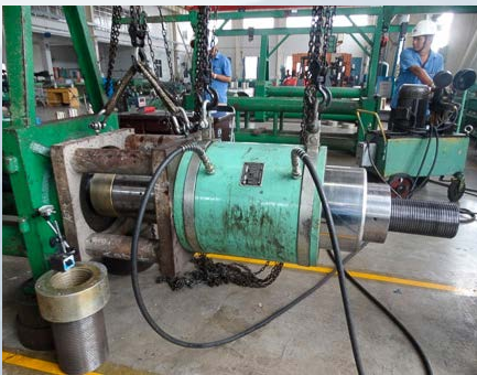
Static load test
