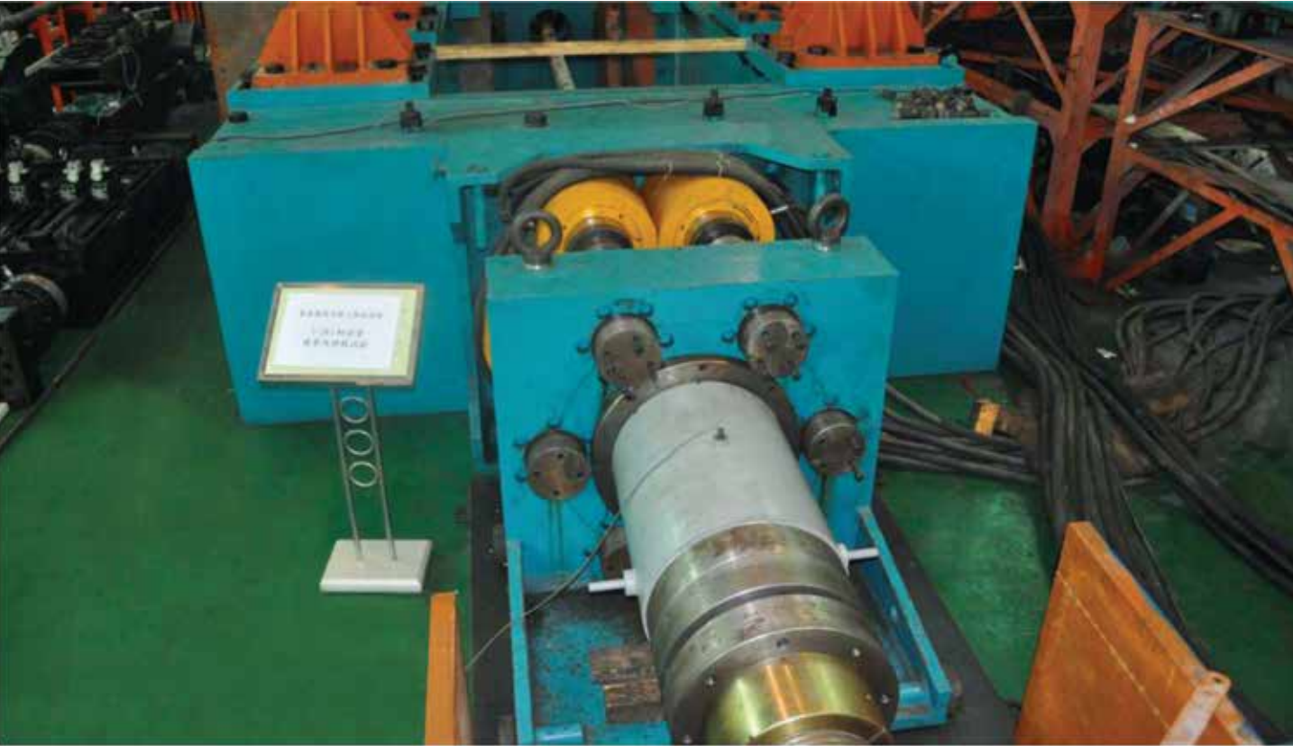
Fatigue and Static Load Test on Type 1670LZM7-283
