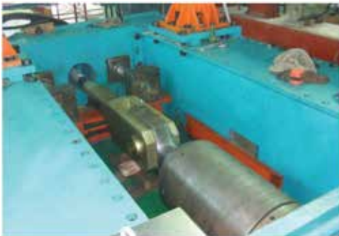
Fatigue Test of 1670LZM7-283 Fork
