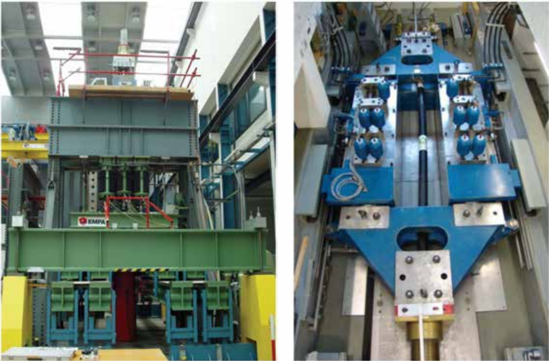
Fatigue and Static Load Test of Type 1670LZM7-211
