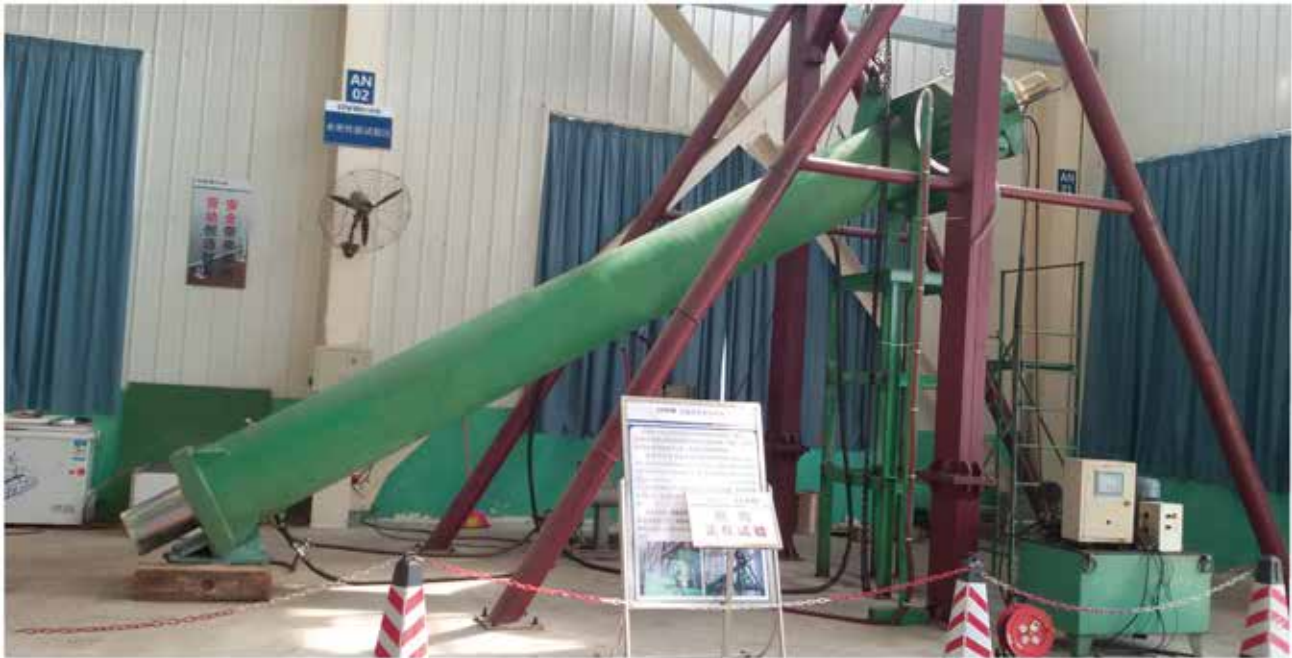
Water tightness test of stay cable (CIP)
