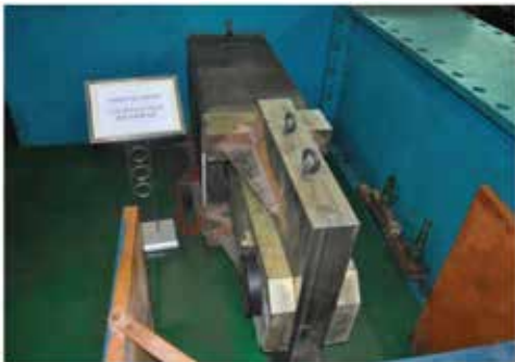
Static Load Test of 1670LZM7-283 Fork
