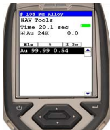
Figure 3. Based on factory calibration, results of analysis of unknown samples are displayed
