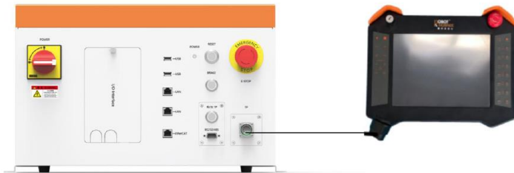
Figure 4-3 Teach Pendant connection diagram
