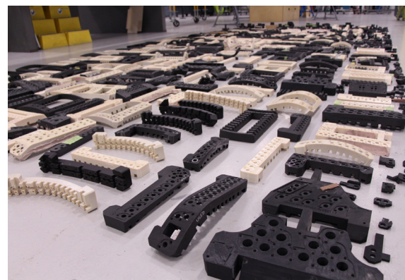
A sample of 3D printed drill guides used in the production of the XB-1 demonstrator aircraft.
