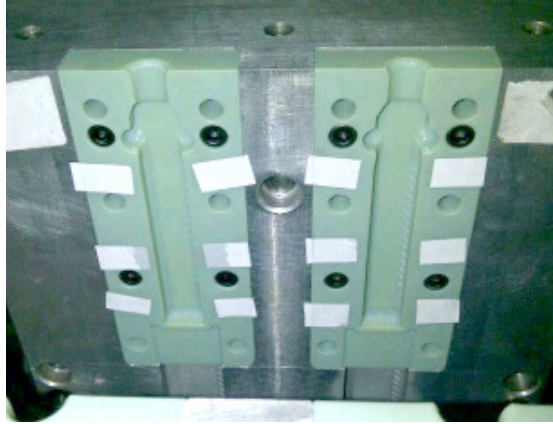
PolyJet printed molds mounted on Plasel's blow molding machinery.
