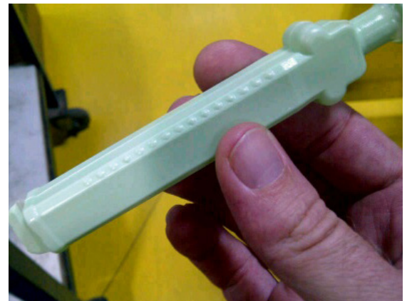
A PolyJet mold was used to produce 100 blow molded package prototypes.
