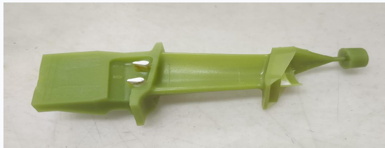
3D Print Sillicore - In the WAX mold
