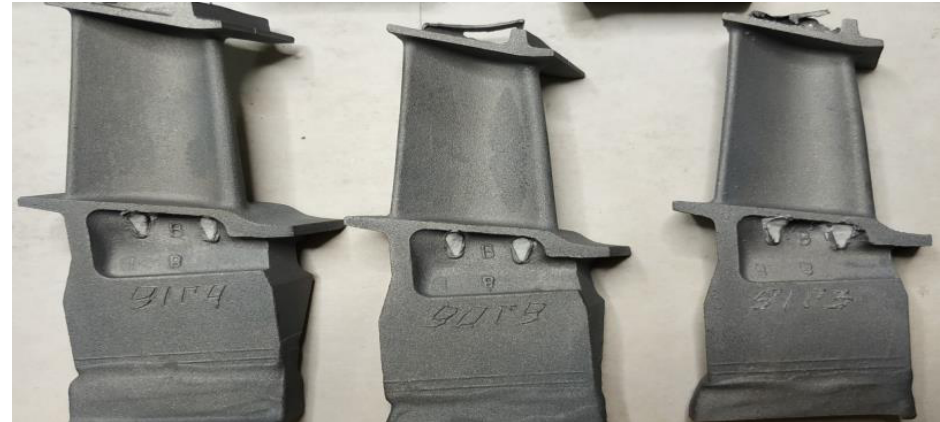
Foundry moulds (Ni-alloy with Silicore cores).
