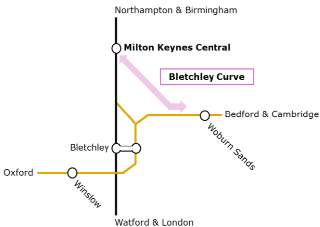
Figure 19 – plan showing EWR services to Milton Keynes with addition of Bletchley Curve enabling access from the east
