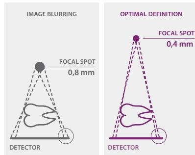
Sharp images at all times RX DC - HyperSphere technology provides your surgery with optimum X-ray quality whatever the type of sensor connected. Now even more powerful, with 70 kV and 8 mA, even more flexible and suitable for all commercially available sensors. The constant potential head tube, associated with the smallest intraoral imaging focal spot available (0.4 mm), ensures the best images whatever your diagnostic needs.
