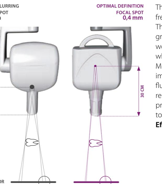
The DC generator in the head tube is high-frequency and constant-potential. This technology gives sharp images with greater detail and lower exposure times than would be attainable with AC X-ray units, which are characterised by variable emissions. Moreover, constant-potential design ensures image generation is unaffected by power fluctuations. RX DC - eXTend technology is reliable for all diagnostic needs and always provides high-definition images by adapting to the sensor type.
