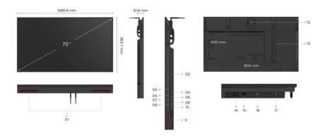
1. Speaker 8. HDMI 2 15. Power Switch 2. OPS Slot 9. HDMI OUT 16. LAN 3. USB 2.0 10. HDMI 3 17. SPDIF 4. RS-232 11. Control Panel 5. USB 3.0 12. WiFi Slot 6. USB-C 13. VESA® Wall Mount (800x600mm) 7. HDMI 1(ARC) 14. AC IN
