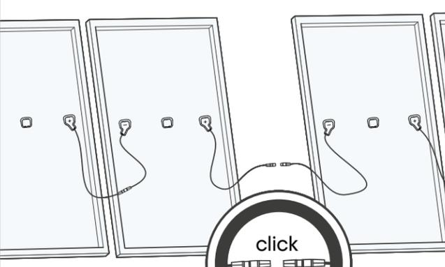
**!** → Do not connect modules with different orientations or angles of inclination in the same string.
