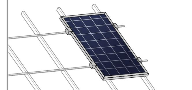
→ Maintain an interval of at least 0.39 in (10 mm) between two modules along the short side and 0.20 in (5 mm) along the long side.
