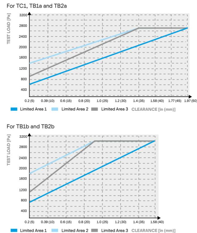
**Fig. 4:** Push loads in relation to minimum clearance between frame bottom edge and substructure.
