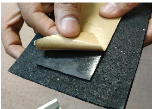
Fig. 6 – Peel mask off tape
