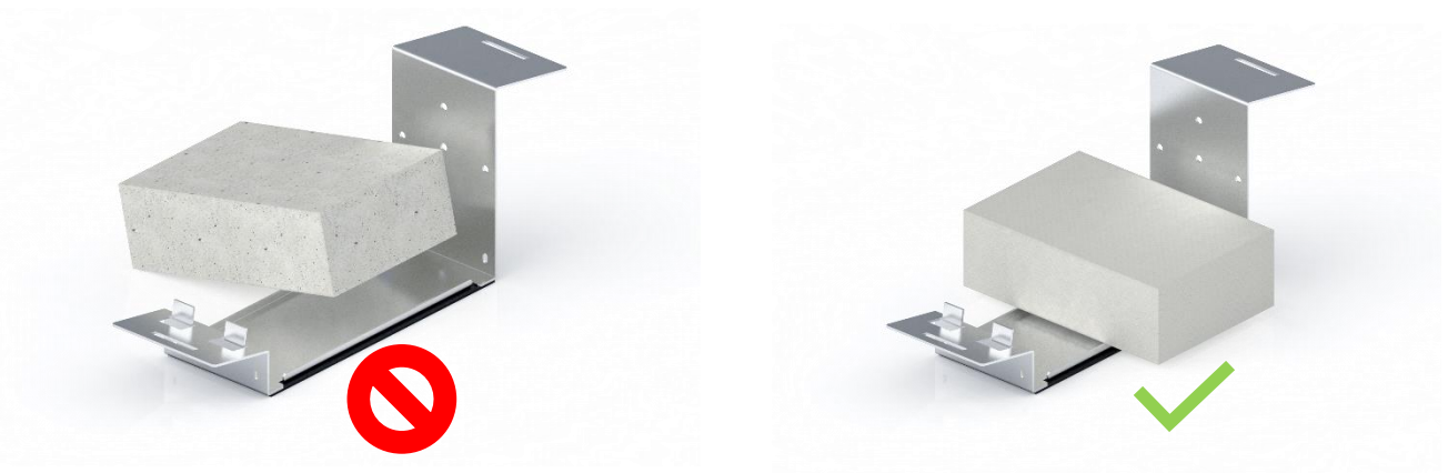
Fig. 5 - Place ballasts with majority of their weight on the support
