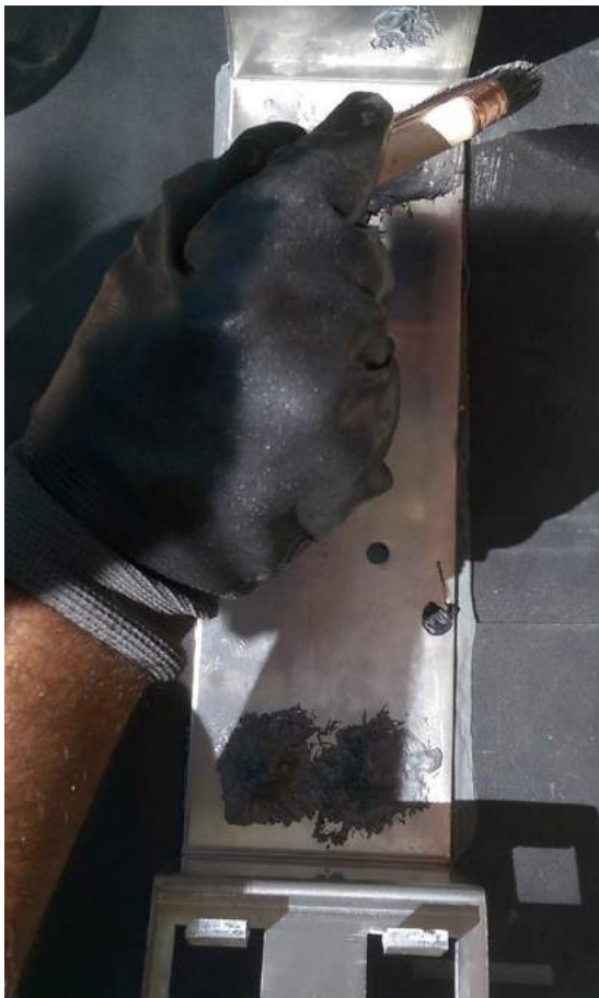
Figure 7 - Step 8: H.E.R Sealant painted on screw heads
