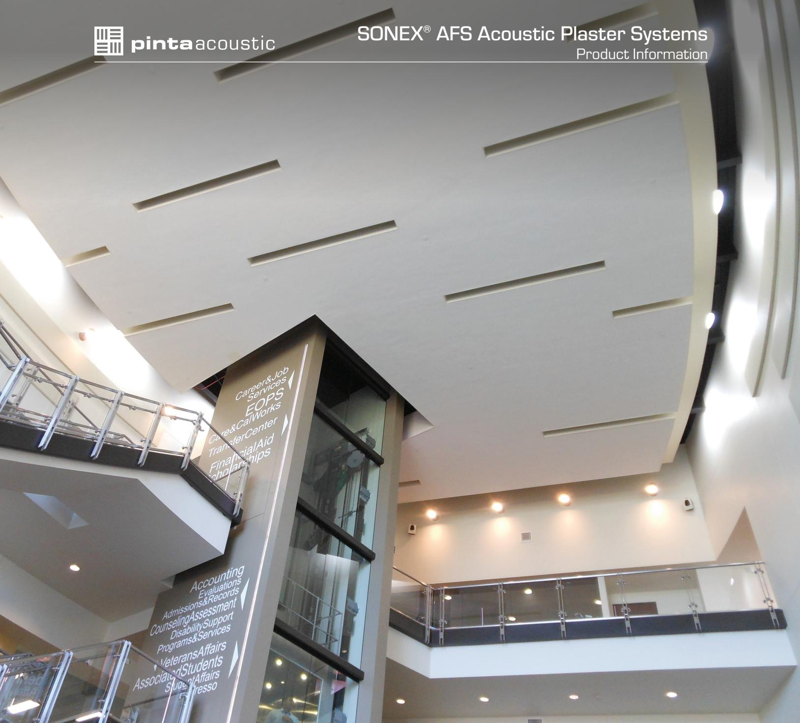
Providing a seamless look, SONEX AFS is typically adhered to gypsum substrates. SONEX AFS consists of single- or double-sided fiberglass mesh laminated to WILLTEC™ open-cell melamine foam panels. Joints between panels are taped and finished. Then base and finish coats of PA-85 plaster are trowel applied, creating smooth monolithic walls or ceilings. Sound energy travels through the acoustically porous finish and gets absorbed into the WILLTEC panel, delivering exceptional NRC ratings.
