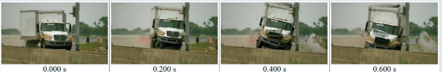
Time-lapse of MASH 4-12 (TL-4) crash test
