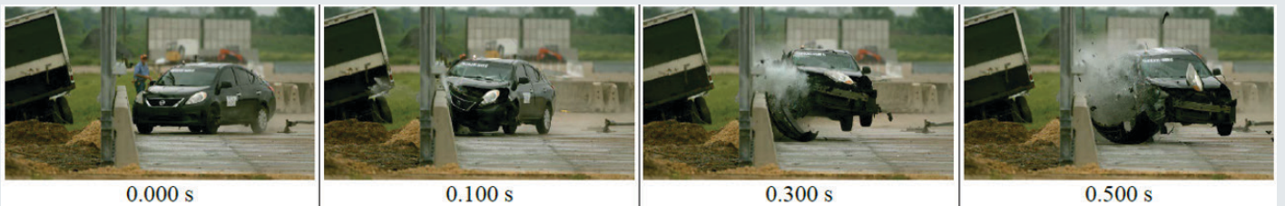
Time-lapse of MASH 4-10 (TL-2) crash test
