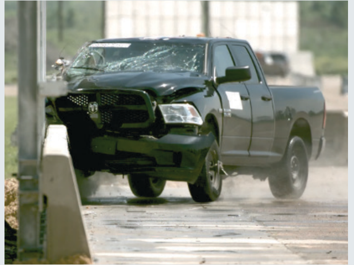
Still image of the heavy duty pick-up truck used in the TL-3 MASH Crash Test at Texas A&M Transportation Institute Proving Ground, College Station, TX.
