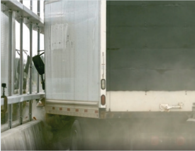
Still image of the box truck used in the TL-4 MASH Crash Test at Texas A&M Transportation Institute Proving Ground, College Station, TX.
