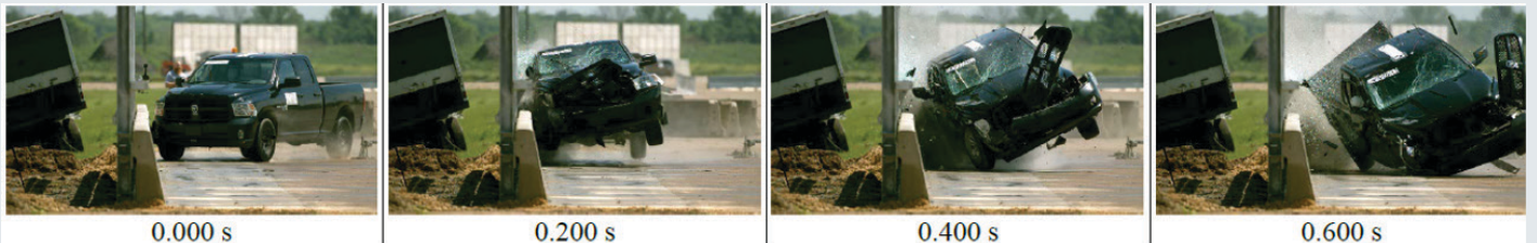
Time-lapse of MASH 4-11 (TL-3) crash test
