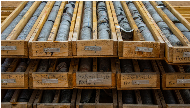
Core Boxes Containing Rock Samples
