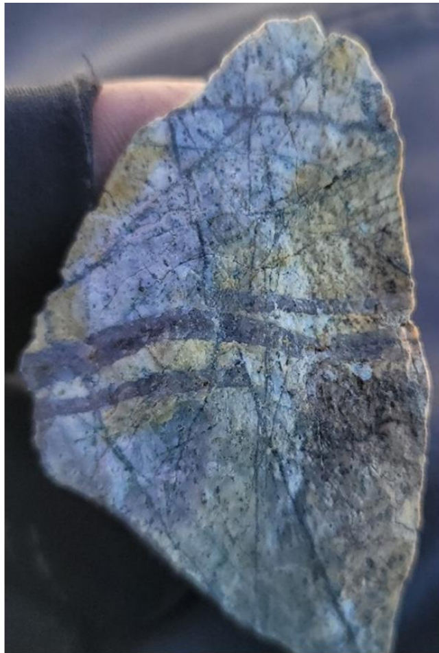
Cuenca: structurally controlled zones of fine "A" type veins crosscut by irregular sheeted veining with incipient development of mid rib to vein, characteristic of porphyry style "B" veins. Overprint of argillic to advanced argillic alteration. Anomalous Au Ag Sb As (Cu Zn Pb) rock chip assays
