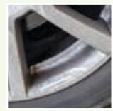
BRAKE DUST STAINING
