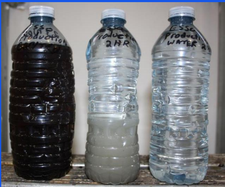
Production water: High silica removal, hardness reduction, immediate sludge flocculation
