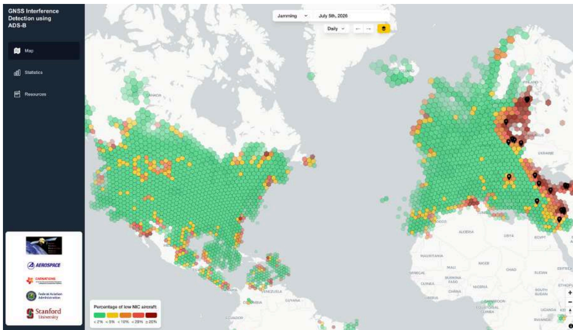
Figure: Map of identified spoof events and ADS-B locations (before spoofing) relevant to the RFI from rfi.stanford.edu
