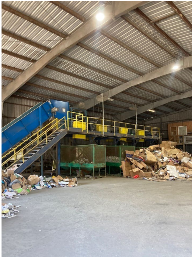
Figure 48: Georgetown County MRF Sorting Line
