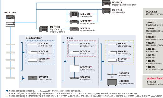
1: Up to three MX-MS10 and/or MX-TR22 can be configured without installing an MX-FN38. 2: Requires Caster Base. 3 When installing a Spacer, install it first, and then install any optional trays above it.
