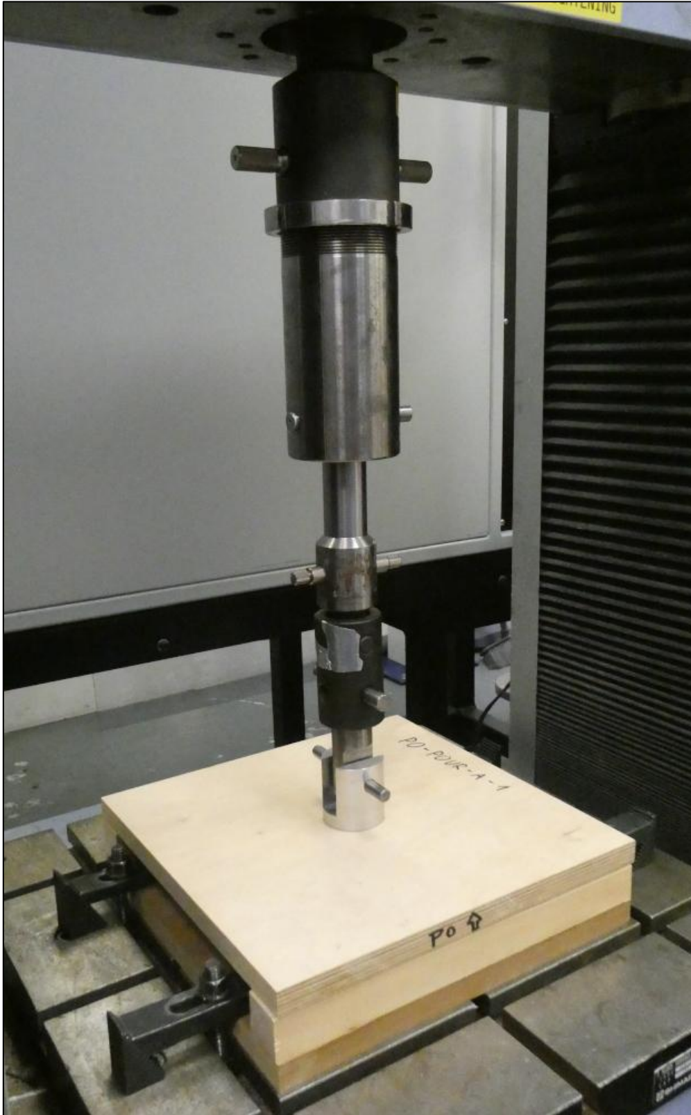
Figure D1 – Pull Off Test Setup
