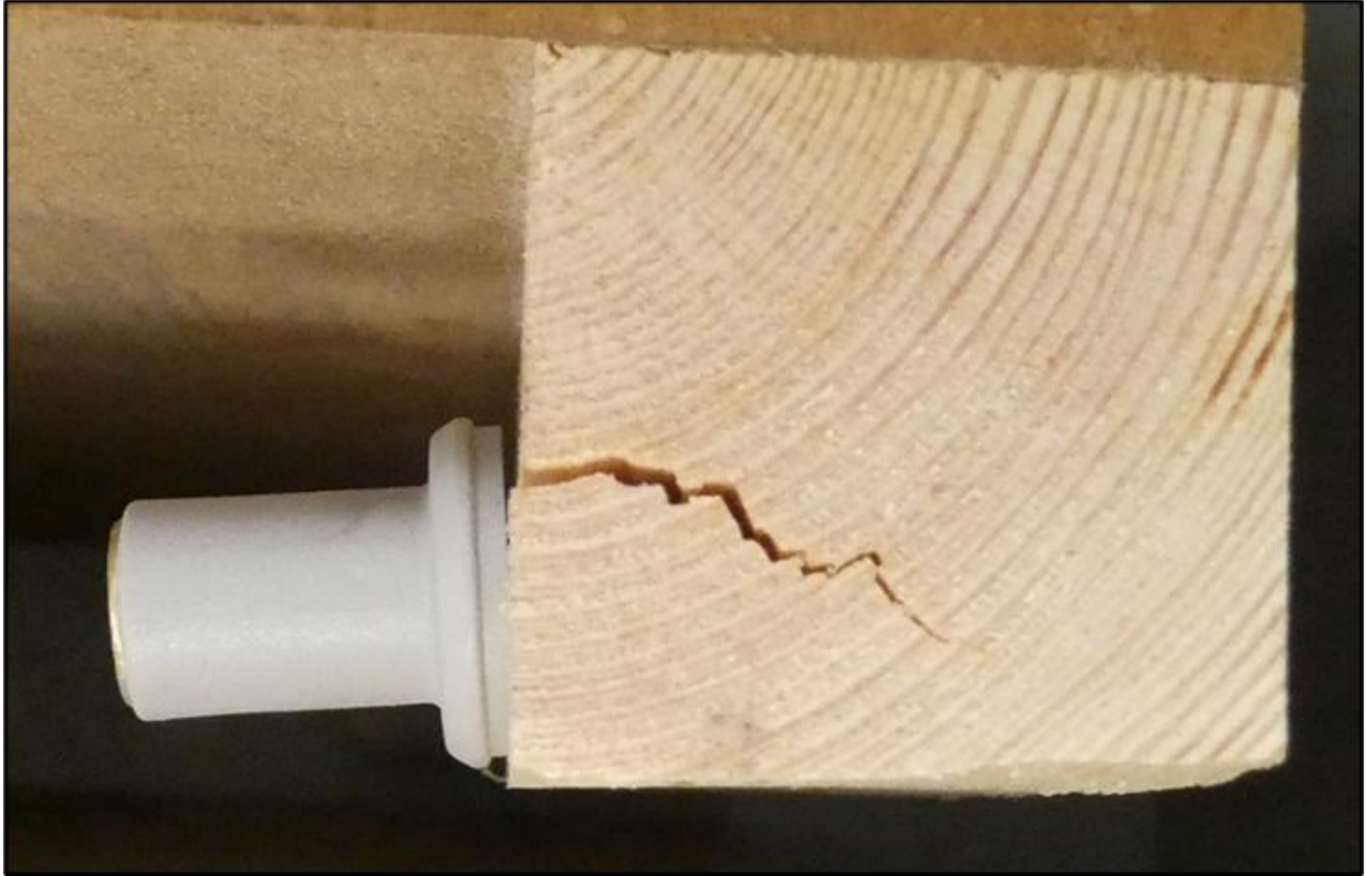
Figure C3 –Drop Down Fixing Pull Off Cracked Batten
