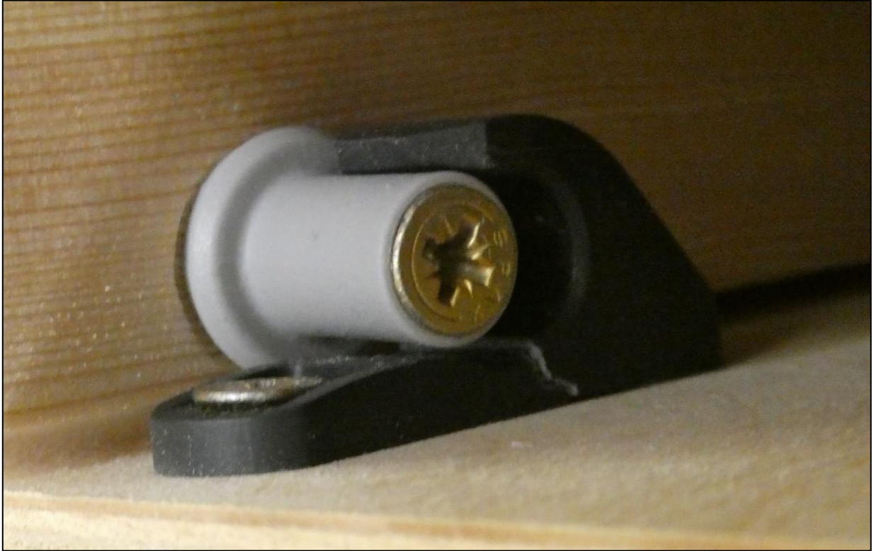
Figure C5 –Drop Down Fixing Shear Failure Modes Example
