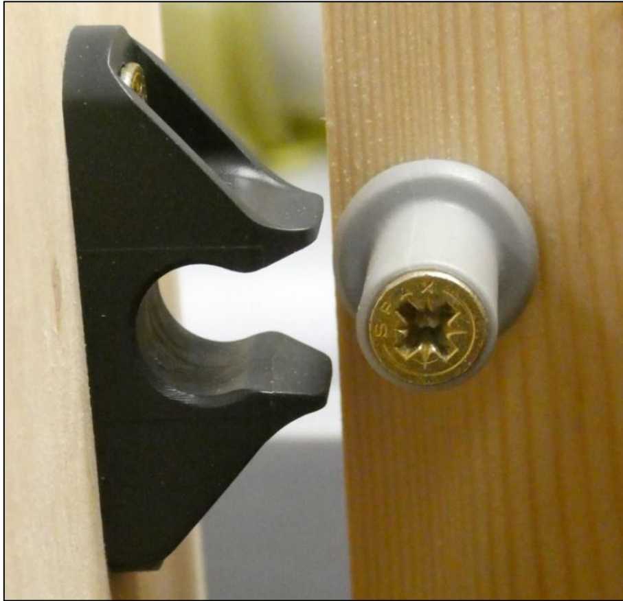
Figure C1 – Push-on Fixing Pull Off Failure Modes Example
