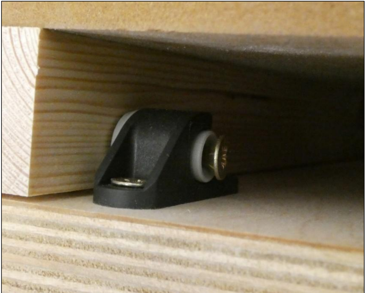
Figure C6 –Drop Down Fixing Shear Failure Mode Pulled Out Screw
