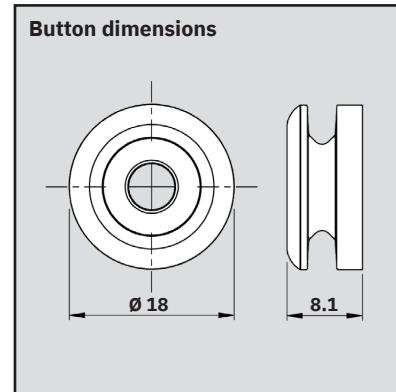
**Material:** ABS (Fix) & Nylon PA6, 30% glass filled
