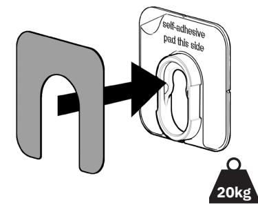
**Abrade surface with emery cloth and clean with isopropyl alcohol**
